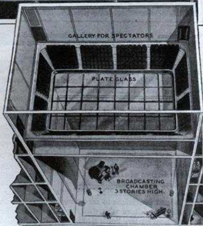
Broadcasting chambers three stories high, entirely enclosed with plate glass and surrounded with galleries for spectators, as shown here, will be provided in the new Radio City.
